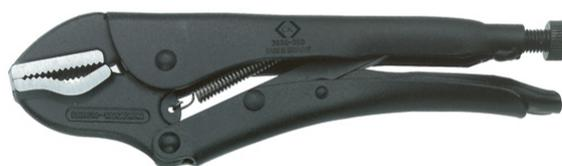
**Features & Benefits** ~ Forged chrome vanadium jaws for strength & durability ~ Combination straight & curved jaws ideal for gripping round, flat & square profile ~ Epoxy coated for corrosion protection ~ Quick release lever ~ Capacity: 35 mm ~ Length: 250 mm
