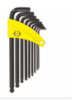
$\sim$  Chrome vanadium steel, hardened & tempered for strength & durability  $\sim$  Ball ended for use at an angle of up to 25° where access is restricted  $\sim$  Supplied in a storage holder  $\sim$  Contents: 5/64[], 3/32[], 1/8[], 5/32[], 3/16[], 7/32[], ü[], 5/16[] und 3/8[] Features & Benefits
