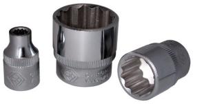
Features & Benefits ~ Forged Chrome Vanadium steel for superior strength & durability ~ Non slip, satin chrome plated for resistance to rust & peeling ~ C.K Sure-drive system applies torque to the flat of the nut rather than the corners to avoid rounding off ~ Drive: 1/2\" ~ Size: 10 mm
