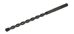
$\sim$  Tungsten carbide tipped with optimized geometry for drilling concrete and stone  $\sim$  Vacuum brazed tips for durability  $\sim$  Ground flutes designed for optimum debris removal  $\sim$  SDS-plus shank  $\sim$  Diameter: 20 mm  $\sim$  Working length: 250 mm  $\sim$  Total length: 310 mm Features & Benefits
