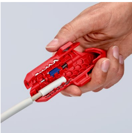
Stripping of a NYM cable
