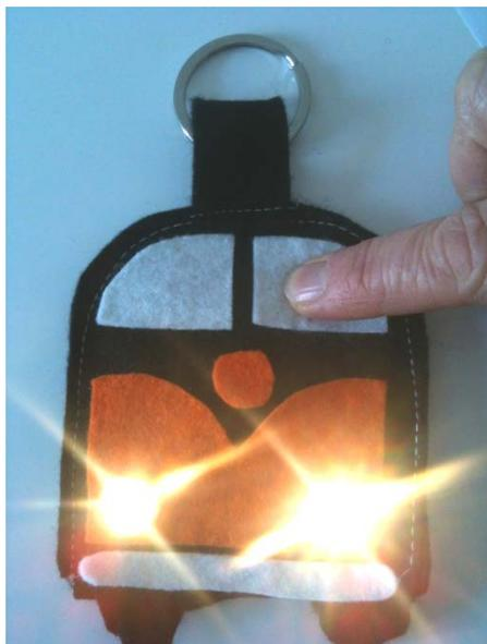
You will see that when the soft pad is pressed in the camper van window, it acts as a switch to turn the van lights on!
