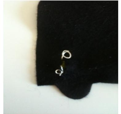
**4.** Knot one end of the conductive thread onto the negative hole on the battery holder. Make sure the knot is tied securely.
