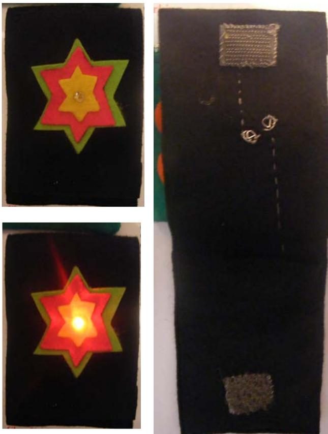
Conductive Hoop & Loop (Velcro™) can be used as a switch, it works in exactly the same way as the press stud. As explained earlier in Diagram 3.
