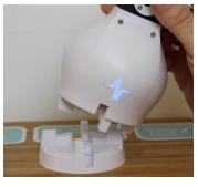
Turn on the Joint module by sliding the switch on the back. Notice that the Joint module has a "name" - this one is called PCA. Remember your Joint module's name.
