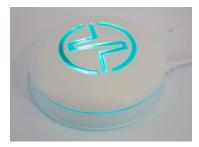
Once connected, the Hub will light up. This should be the same color as the Joint module. If it isn't, press either the Hub or the joint module until they have the same color.
