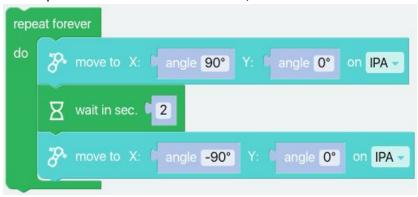
Now, the Joint module will continuously move from 90 to -90 degrees.
