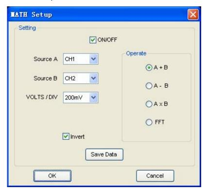
**ON/OFF**: Turns the MATH Channel On or Off. **Source A/B**: Set the sources of the math channel.
