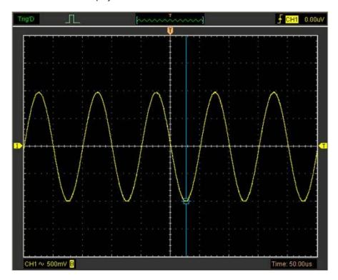
The **Trace** cursor measurement result is displayed on the status bar.
