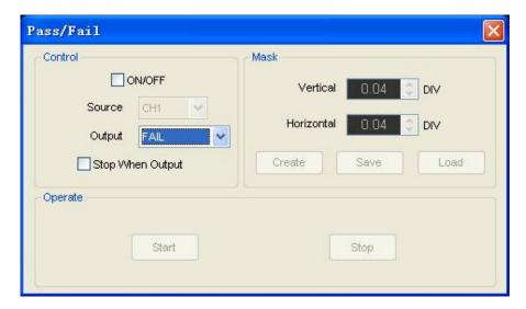
The **Pass/Fail** function monitors changes to the signals or the outputs by comparing the input signal with a pre-created template.
