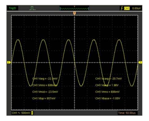
**Note**: The results of the automatic measurements will be displayed on the bottom of the screen. A maximum of 8 results can be displayed at the same time. When there is no room, the next new measurement result will make the previous results move left, off of the screen.
