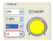
**Note**: The attenuation factor changes the vertical scale of the oscilloscope so that the measurement results reflect the actual voltage levels at the probe tip.
