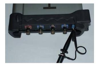
2. Set the CH1 probe attenuation of the oscilloscope to x10. (The default is x1).
