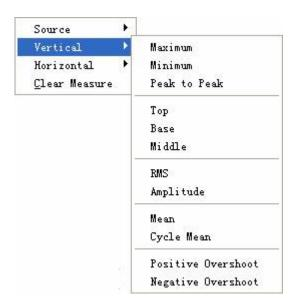
Maximum: Voltage of the absolute maximum level, Measured over the entire waveform
