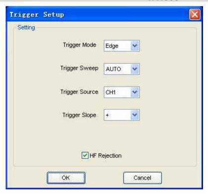
The user can turn on "HF Rejection" to eliminate triggering higher-frequencies. (20M above).
