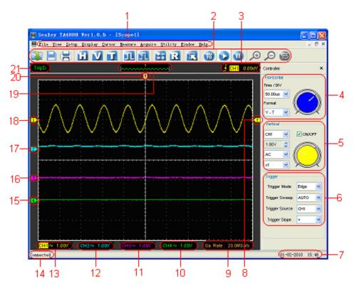
In addition to displaying waveforms, the display area shows additional information about the waveform and the oscilloscope control settings.
