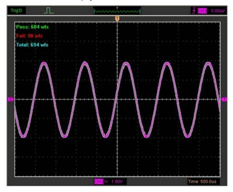
NOTE: Pass/Fall function is unavailable In X-Y mode and Roll mode.
