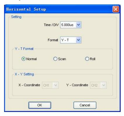
1. Time/DIV: Allows the setting of the time base parameters
