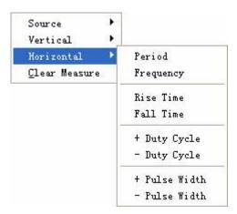
**Period**: Time to take for the first signal cycle to complete in the waveform
