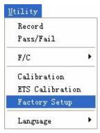
When you click the **Factory Setup** in **Utility** menu, the oscilloscope displays the CH1 and CH2 waveforms and removes all other waveforms.
