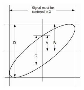
$Sin\theta = A/B \text{ or } C/D$ , where  $\theta = phase shift (in degrees) between the two signals.$
