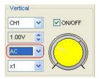
You can set the coupling to **DC**, **AC** or **GND**. If you set the coupling to **DC**, it blocks the **AC** component of the input signal.
